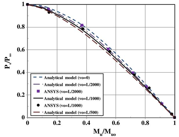
Fig. 9. Comparison between the interaction diagram obtained from the developed model and finite element non-linear analysis ( $b_f = 150$  mm,  $t_f = 12$  mm,  $d_w = 500$  mm,  $t_w = 10$  and  $L = 6.0$  m),  $M_{u0}$  = Pure bending ultimate capacity (beam),  $P_{u0}$  = Pure axial ultimate capacity (column).
