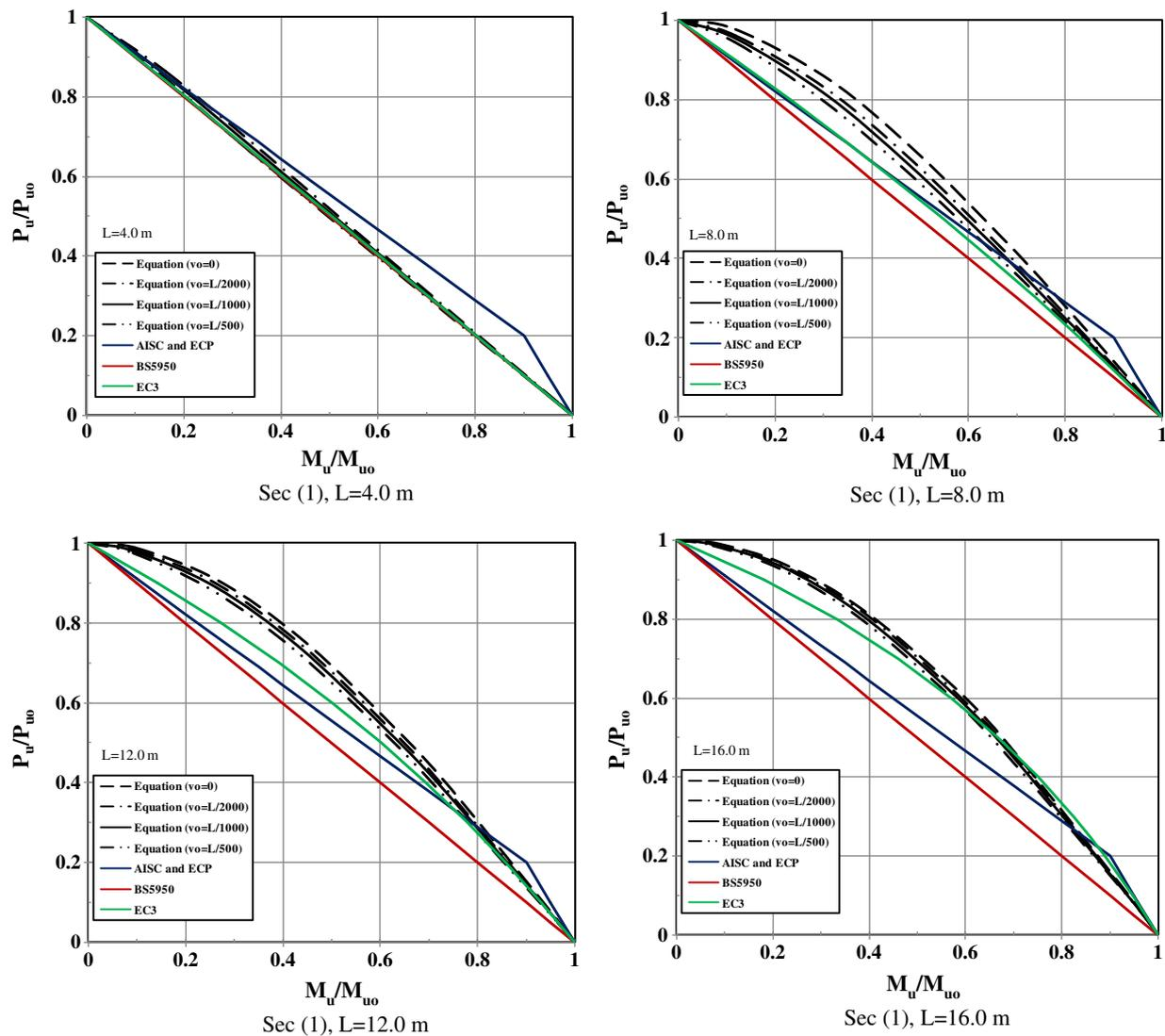
Fig. 11. Comparison between the proposed design method and the design codes methods for the first I-section,  $b_f = 200$  mm,  $t_f = 16$  mm,  $d_w = 600$  mm,  $t_w = 8$  mm,  $L = 4, 8, 12$  and  $16$  m.
