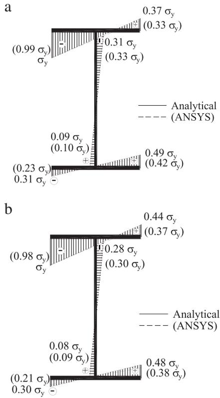
**Fig. 10.** (a) Comparison between stress distribution obtained by analytical solution and finite element analysis ( $v_0 = L/2000$ ,  $e/d_w = 0.5$ ),  $P_u/P_{u0} = 0.63$ ,  $M_u/M_{u0} = 0.53$ . (b) Comparison between stress distribution obtained by analytical solution and finite element analysis ( $v_0 = L/1000$ ,  $e/d_w = 0.5$ ),  $P_u/P_{u0} = 0.61$ ,  $M_u/M_{u0} = 0.52$ .
