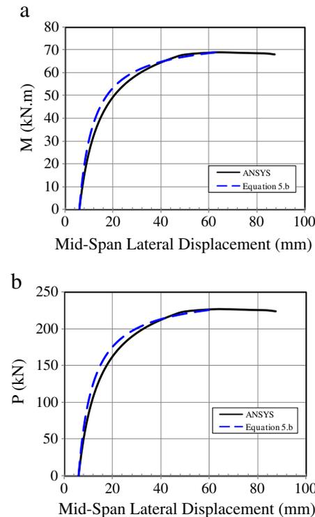
Fig. 8. (a) Moment–displacement curve for  $v_0 = L/1000$ ,  $e/d_w = 0.5$ . (b) Force–displacement curves for  $v_0 = L/1000$ ,  $e/d_w = 0.5$ .
