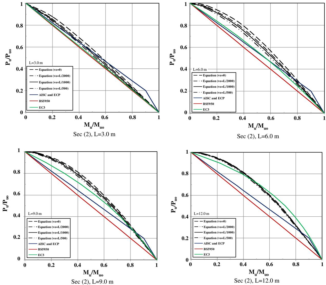
Fig. 12. Comparison between the proposed design method and the design codes methods for the second I-section,  $b_f = 150$  mm,  $t_f = 12$  mm,  $d_w = 500$  mm,  $t_w = 10$  mm,  $L = 3, 6, 9$  and  $12$  m.
