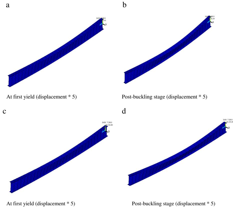
**Fig. 6.** (a) Deformed shape of the second section,  $L = 6$  m,  $v_o = L/2000 = 3$  mm,  $e/d_w = 0.5$ . (b) Deformed shape of the second section,  $L = 6$  m,  $v_o = L/1000 = 6$  mm,  $e/d_w = 0.5$ .
