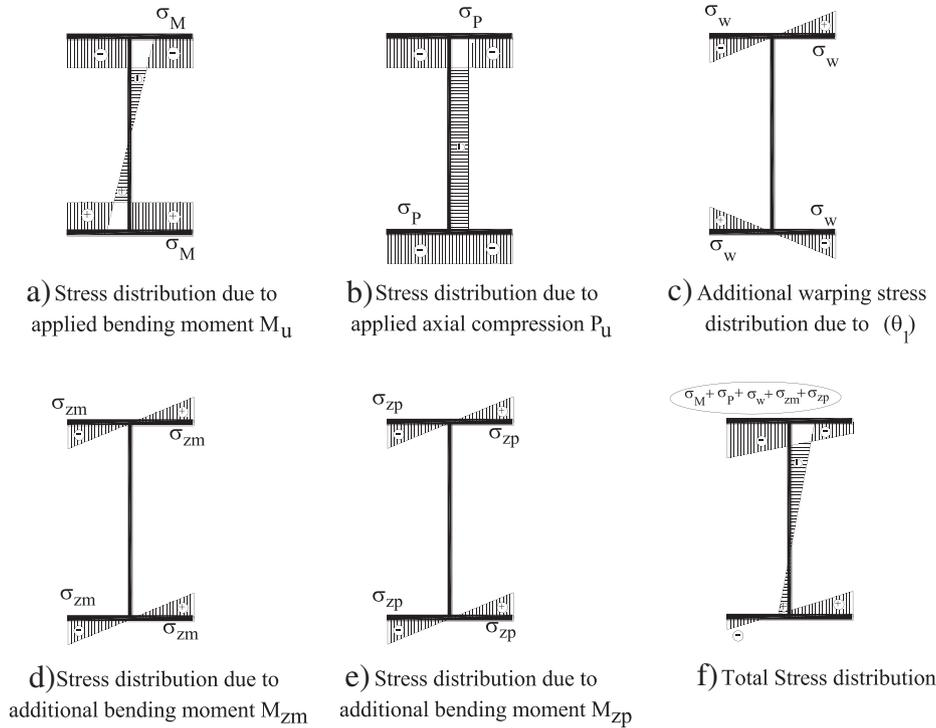
Fig. 5. Stress distribution due to applied and additional straining actions.
