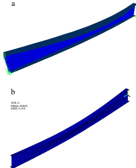
Fig. 2. (a) Buckled shape for first section,  $L=6.0$  m,  $\frac{P_{cr}}{P_{Ez}} = 0.346$ ,  $\frac{M_{cr}}{M_{LTz}} = 0.736$ . (b) Buckled shape for second section,  $L=6.0$  m,  $\frac{P_{cr}}{P_{Ez}} = 0.646$ ,  $\frac{M_{cr}}{M_{LTz}} = 0.535$ .
