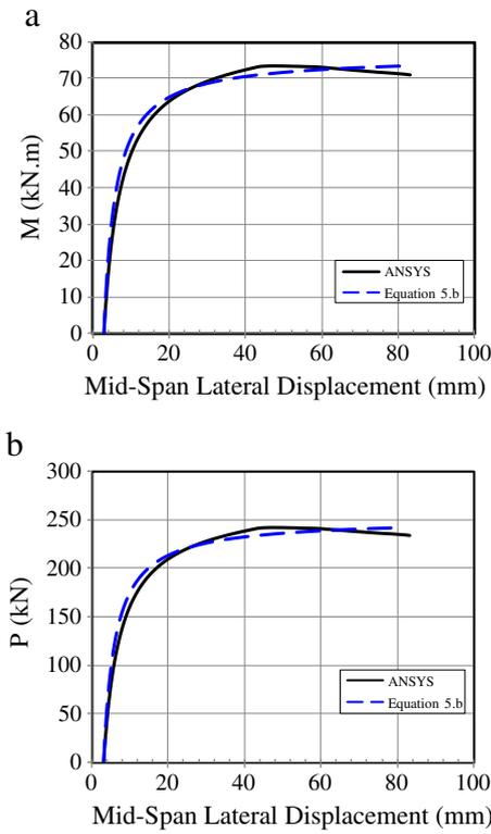
Fig. 7. (a) Moment–displacement curves for  $v_0 = L/2000$ ,  $e/d_w = 0.5$ . (b) Force–displacement curves for  $v_0 = L/2000$ ,  $e/d_w = 0.5$ .
