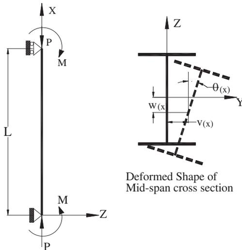
Fig. 1. Beam-column boundary conditions, loads, axes and deformed shape.
