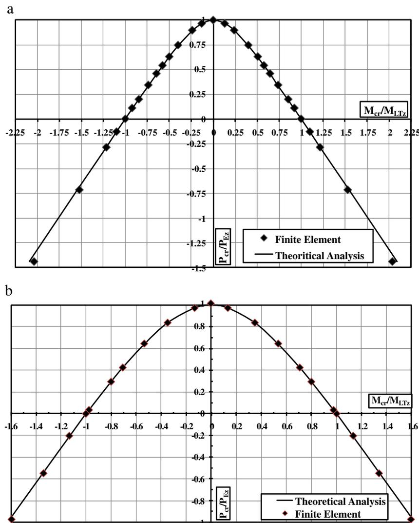
Fig. 3. (a) Comparison between FE and theoretical solution for critical buckling interaction for first section;  $b_f = 200$  mm,  $t_f = 16$  mm,  $d_w = 600$  mm,  $t_w = 8$  mm, and  $L = 6.0$  m. (b) Comparison between FE and theoretical solution for critical buckling interaction for second section;  $b_f = 150$  mm,  $t_f = 12$  mm,  $d_w = 500$  mm,  $t_w = 10$  and  $L = 6.0$  m.
